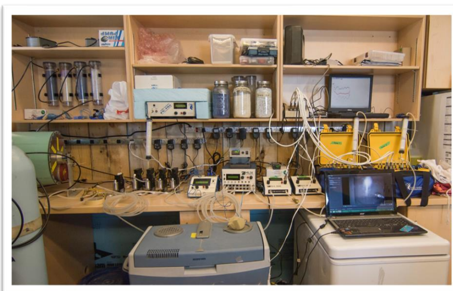
Flow-through respirometry set-up used at Alert to measure the metabolic and evaporative water loss rates of snow buntings (Audrey Le Pogam)
